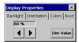
This program can be used to set the backlight to the required value. The setting made is stored as persistent data, i.e. it is retained even after a restart.
